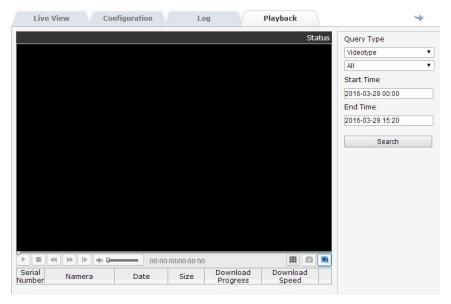
3.5 If cannot find the image or recorder on "playback",check the "Log"if Motion detection is triggered. If not trigger, reset the motion detection. If trigger, check the schedule recorder is set as motion detection type.
