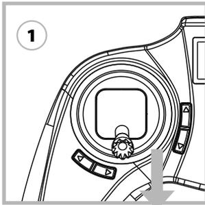
1 Move the transmitter's joystick (and throttle trim) to the minimum throttle setting.
