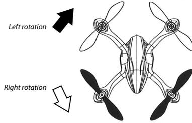
The control lever for Turn turns your quadcopter left/right.
