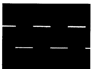
⑳ IC307 ②pin (LRCK) 5.6Vp-p, 5μs
