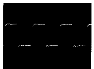
⑱ IC307 ⑦pin (BCK) 5.2Vp-p, 0.1μs
