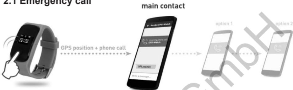
If you press the SOS button for 3 seconds the watch will trigger an emergency call and an emergency SMS. The three emergency contacts will be called one after another until one contact answers the call. If no contact picks up the call, it starts from the beginning with the first emergency contact. This procedure will be repeated up to three times. Also an emergency SMS with the actual position will be sent.
