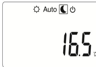
The rated temperature of economy operation is constantly kept at a value that can be set between 5° C and 35° C in steps of 0.5°C.
