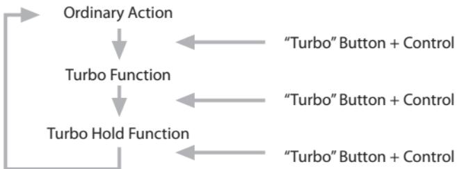
Note: When the WIRELESS Controller is set to Turbo Hold it will enter Sleep Mode after an idle time of three minutes.
