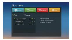
The DISPLAY tab allows you to change the output resolution and is set to auto detect by default. You can also change the display position as carried out in the initial setup (chapter 3.3)
