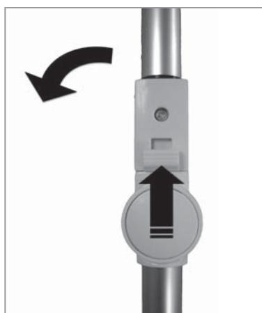
3. You can fold the bar through an angle of up to 90° for better handling: Press in the button on the side of the articulated joint and move the bar in the direction of the battery compartment (see illustration). The angle is continuously adjustable.
