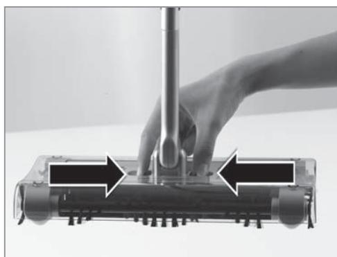
3. Hold the cleaning foot over a waste bin and open the dirt container by pressing together the two locking clips next to the bar (see illustration).
