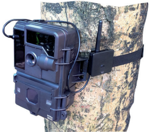
camera model with invisible IR flash - no covering needed
