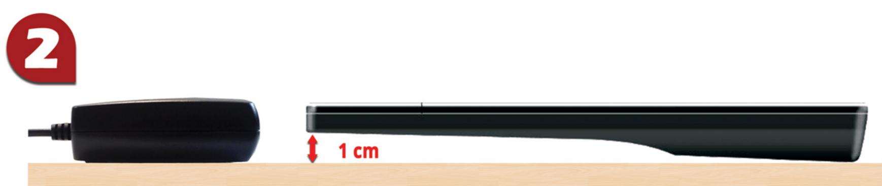
Make sure Usb-Programmer Led and Superior Slim are on the same level: the head of remote control should be around 1cm high from the table.
