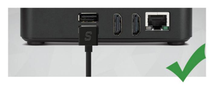
Always connect the Usb-Progammer directly to the usb port of your PC.
