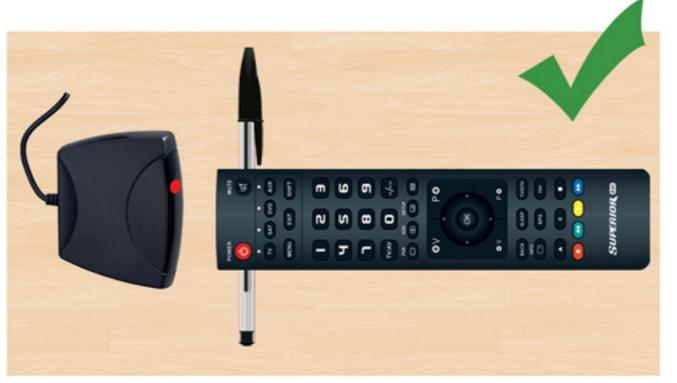
Just place a pen under the Remote Control to easily reach the correct allignment level.
