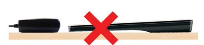
If the head of remote is going down, the remote won't be aligned to the Programmer.
