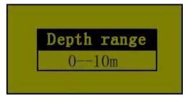
**Water depth range setting:** Press the + or - button to adjust. A proper setting can make the picture more clear. You can also set to AUTO to let the system adjust the parameter.
