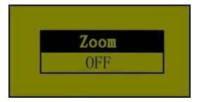
**The bottom zoom display function:** Press + or - to turn it on or off. The user can use this feature to see the details under the water.
