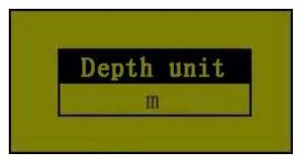
Water depth display unit: Press + for feet, press - for meters
