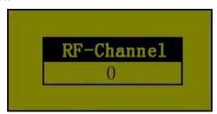
**RF channel selection:**When there are 2 bait boats in the same area, the user should choose different channel by press + or -. The user need to reboot the bait boat to save the change. There are 6 channels available for user to choose.
