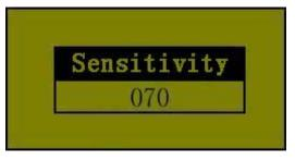
**Sonar detection sensitivity setting:** Press + or - to adjust. When the water is too deep or unclear, the user should increase the sensitivity. The best range should be between 60 - 90. Higher sensitivity level may detect false target.
