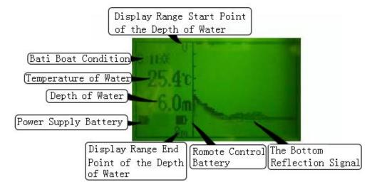
The depth range for this system is 0.6 - 32 meters. The system won't work outside of this range. If the estimated depth is shallow, we can choose low sensitivity. For example, 60 for 5 meters. The deep depth, the higher sensitivity. Try not to set the sensitivity to a very high level, it may cause false target.
