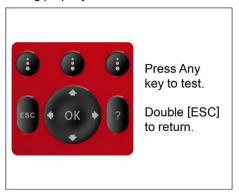
Figure 7-5 Sample Key Test Screen
