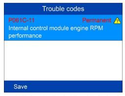
Figure 3-10 Sample Engine Trouble Codes Screen
