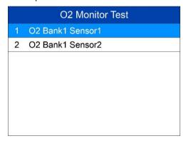
Figure 4-17 Sample O2 Monitor Test Menu
