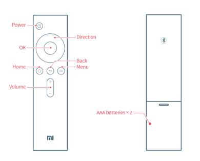
Power: Press to select, Reboot, Power Off 20 sec, Delayed Power Off, Screen off options.
