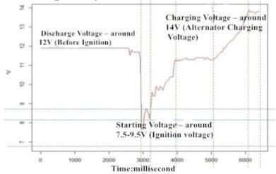
Left side: Discharge Voltage – around 12V (Before Ignition) Mid:Starting Voltage – around 7.5-9.5V (Ignition voltage) Right: Charging Voltage – around 14V (Alternator Charging Voltage)
