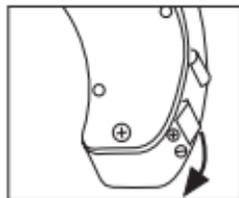
2. Remove the protective film from the button cell battery included in delivery (type 13/PR48) and insert the battery into the battery compartment as shown after 10 to 15 minutes. When inserting the battery, ensure that the correct polarity (+/-) is observed.
