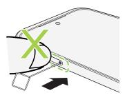
3. Push the tip into the hole until the tray ejects, and then pull the tray out.
