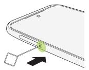
When inserting the eject tool into the tray eject hole to remove the card tray, do not obstruct the tray to avoid damaging the eject mechanism inside the slot.
