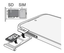
When you need to use a second nano SIM card, remove the microSD card and place the nano SIM into the outer holder. You cannot have the second nano SIM and microSD cards inserted at the same time.
