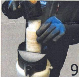
*Then mount the filling funnel with a short sharp blow on the container. To ensure a uniform pressure distribution of the shock during installation, we recommend using a suitable edition (Mounting bolt ref.no. 977144.0000 or a wooden board).*
