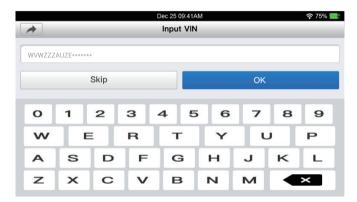
Input the VIN, and tap "OK", the system will decode the VIN data automatically, and continue the Smart Diagnosis procudure if success. Otherwise the system will enter the Manual Diagnosis mode.
