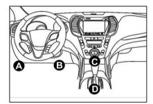
3. Plug the diagnostic cable into the vehicle's DLC socket.
