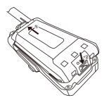
Insert the top part of the battery pack into the top 2 slots of the transceiver and then press the battery pack down until a "click" sound is heard.
