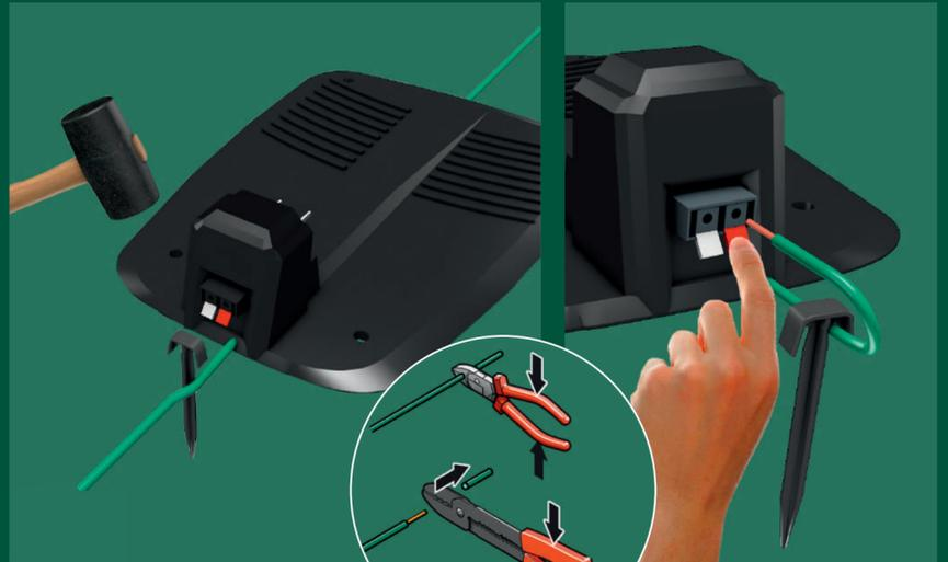
**EN:** Peg the wire 10 cm away from the docking station. Strip 10–15 mm of insulation off the wire. Then connect the wire to the right hand (red) terminal. Do not peg the wire fully down but leave 2 cm of peg sticking out until Step 8.
