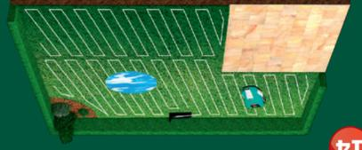
**EN:** Once the lawn area has been mapped and learned, the Indego is able to efficiently navigate around the lawn, cutting the grass in parallel lanes and avoiding objects before returning to the docking station.
