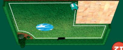
**EN:** During setup the Indego will map the lawn area and save its shape to memory. To do this, it will drive around the edge of the lawn area recording how far it has travelled. Once completed, the Indego is ready to cut the grass. Note: during mapping the Indego will only follow the outer perimeter wire. Do not lift or interrupt the Indego during steps 12 and 13.
