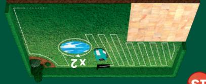
**EN:** During the first two cutting sessions, the Indego will learn the location of the objects within the garden. During this process the Indego will drive around an object to map its shape, then drive to the edge of the cutting area in order to save its location within the lawn map. This process will be repeated a number of times to confirm the location of objects within the lawn area.
