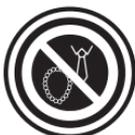
**DO NOT WEAR LOOSE CLOTHING OR JEWELRY WHEN WORKING ON AN ENGINE. Loose clothing can easily be caught in the engine's fan, pulleys, belts, etc. and jewelry is highly conductive, which causes severe burn or electric shock if it contacts with electricity.**
