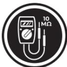
**ALWAYS USE A DIGITAL MULTIMETER WITH AT LEAST 10 MEGOHMS OF IMPEDANCE when conducting electrical tests on vehicles to prevent causing damage to on-board electronic components.**
