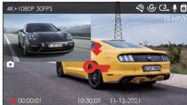
You can set the G-sensor Sensitivity values of Forward & Backward, Leftward & Rightward, Upward & Downward of the car. The G-sensor value in each direction can be selected 1/2/3/4/5/OFF. The default sensitivity for the three dimensions is 3. The highest sensitivity of the G-Sensor is 5. Event videos are stored in the "Video/Event" folder, and cannot be automatically overwritten.
