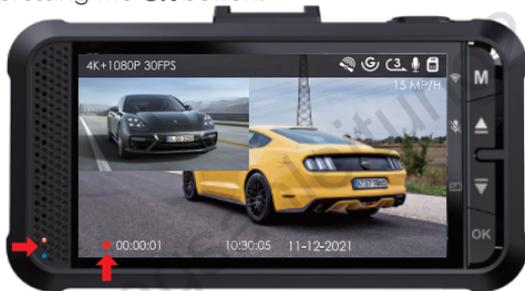
By default, the Loop Recording Time is 3 minutes. Please go to "Record Setup" ► "Loop Recording" to change it to 1 min, 2 mins, 3 mins, 4mins or 5 mins for your need.
